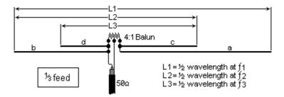
The bands must be twice the frequency of the previous band with this method. For example, if a=60 meters and b=30 meters, then a+b will resonate at about 1.8 MHz. If c=15 meters then b+c will resonate at 3.5MHz. If d=7 meters, then c+d will resonate at about 7 MHz. This technique can reduce the amount of wire you have to buy.
