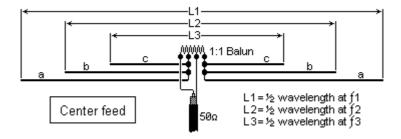
The balun shown above is required to match the ballanced antenna to an unballanced feeder. Typicaly 5 + 5 + 5 turns of thick enamelled wire are wound on a ferrite ring, the three coils are connected in series from the start of one winding to the end of the next. L1, L2 and L3 are for resonance on three different bands. L1 (a+a), L2 (b+b) and L3 (c+c) are equal to:
