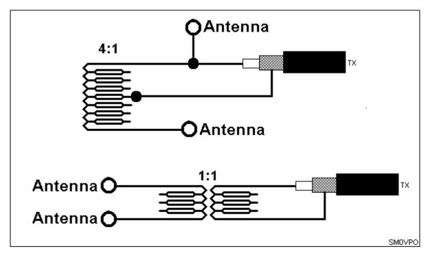
Here you see two methods, the first is a simple AUTO-TRANSFORMER. The RF voltage is doubled and ballanced about a center point. This method will increase the antenna feed impedance by four so with a 50 ohm feeder it is suitable for driving 200 ohm impedance antennas, such as folded dipoles. The second method is simple transformer isolator - crude but effective.
