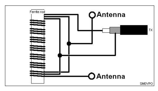
Here we see the same balun wound on a bit of ferrite from an old transistor radio set. This will also work well but the power handling capacity may be reduced a little.
