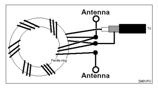
Here we see three pieces of wire twisted together and coiled upon a ferrite ring. This method enables you to have a 1:1 impedance ratio for feeding low impedance antennas such as half-wave HF antennas. This transformer balun has a very wide bandwidth and is suitable throughout the complete HF spectrum. The transformer may be almost any ferrite ring for up to 50 watts or so.
