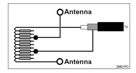
By tapping the coil it is possible to achieve a 1:1 impedance ratio and improve the effect of the second crude method. In practice each winding will be identical to all the others and this can be achieved by twisting together two insulated wires and wrapping a few turns round a bit of ferrite.
