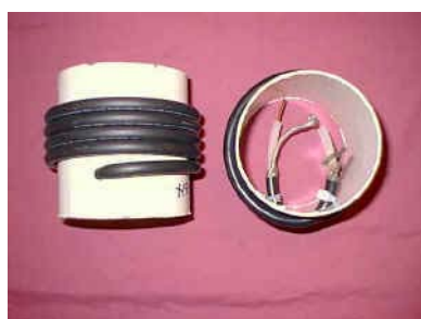
Trap Coil and Wiring
