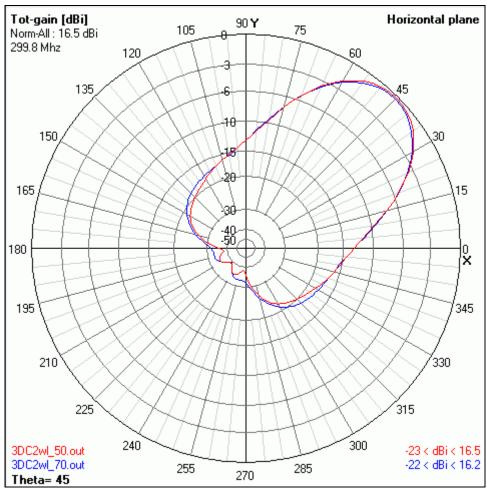
Fig. 8. Horizontal diagram of original and modified 3D Corner Reflector Antene with 2 wavelengths reflector length.
