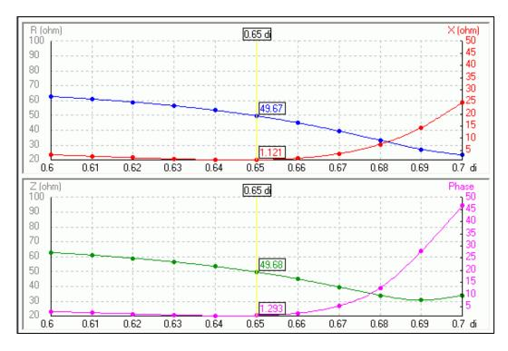
Fig. 12. Modified antenna input impedance change with change of passive element DI length and constant length of active element DR=0.75 wavelengths.
