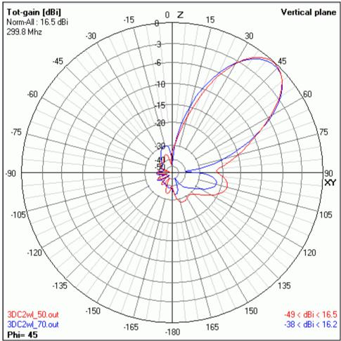
Fig. 7. Vertical diagram of original and modified 3D Corner Reflector Antene with 2 wavelengths reflector length.
