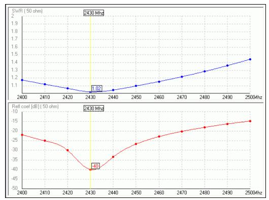
Fig. 27. Input matching and bandwidth of shortened antenna.
