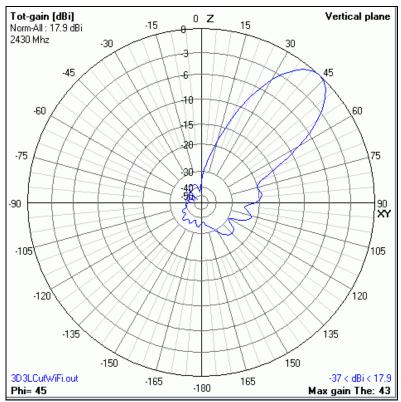
Fig. 21. Vertical diagram of shortened antenna at 2.4 GHz.
