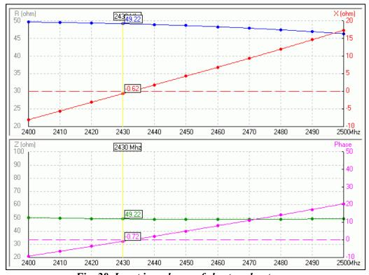
Fig. 28. Input impedance of shortened antenna.
