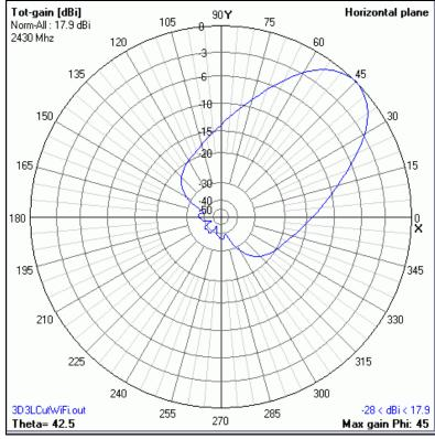
Fig. 22. Horizontal diagram of shortened antenna at 2.4 GHz.
