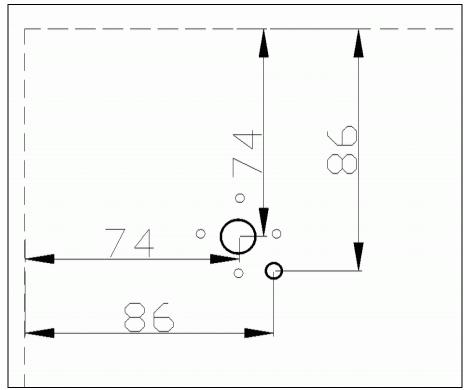
Fig. 30. Dimensions and position of holes for active and passive elements.
