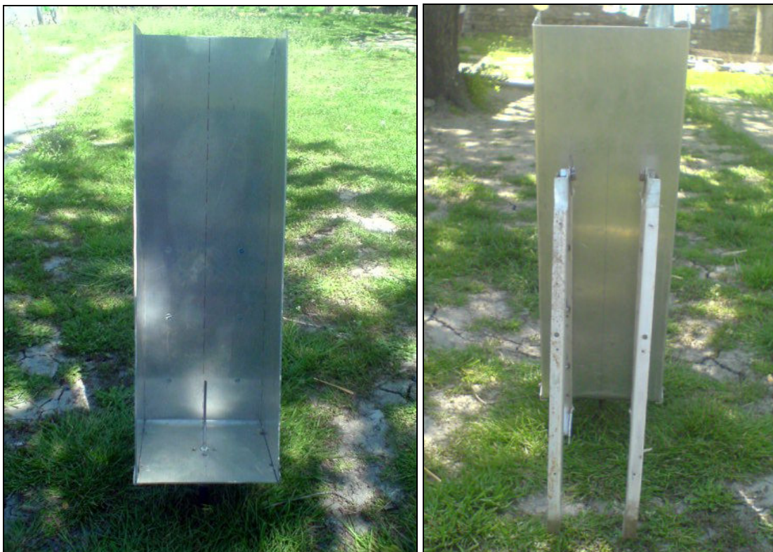
Fig. 21. Obelisk antenna for 2.4 GHz made of aluminium with mounting accessories.
