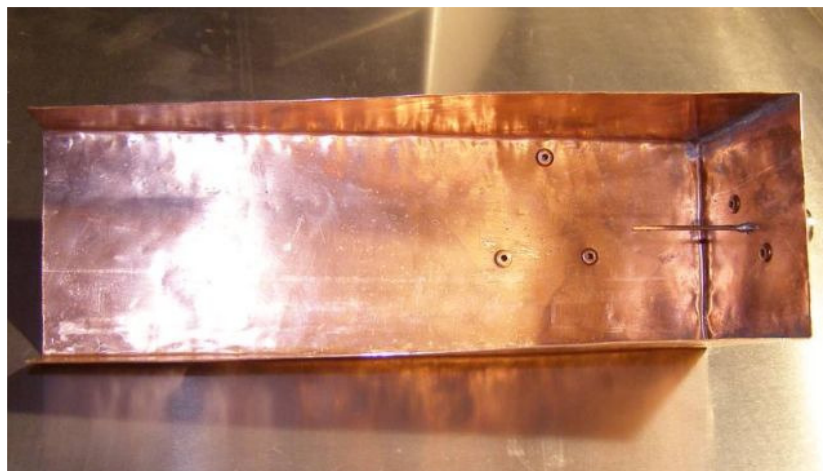
Fig. 19. Obelisk antenna for 5.8 GHz made of copper.
