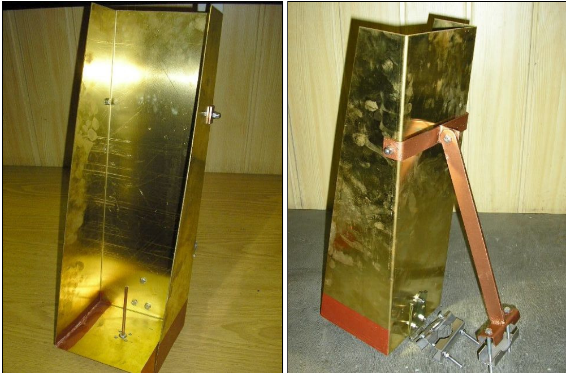
Fig. 20. Obelisk antenna for 2.4 GHz made of brass with mounting accessories.
