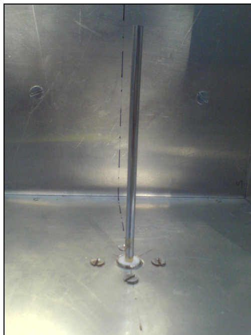
Fig. 22. Obelisk antenna for 5.8 GHz made of aluminium.
