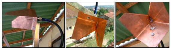
Fig. 20. Outlook of Truncated 3D Corner Reflector Feed mounted in focus of offset parabola
