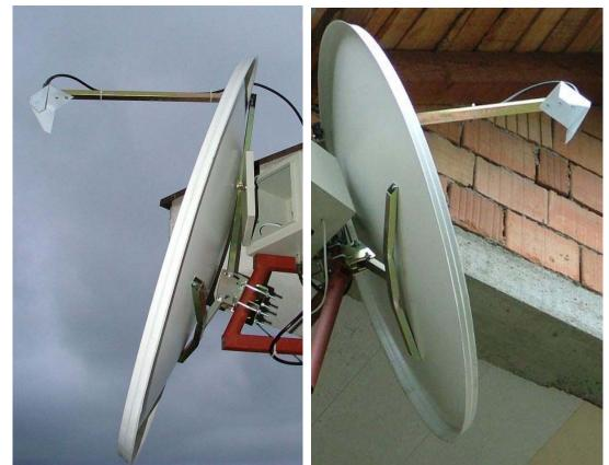
Fig. 19. Practical use of Truncated 3D Corner Reflector Feed with SAT TV offset parabola
