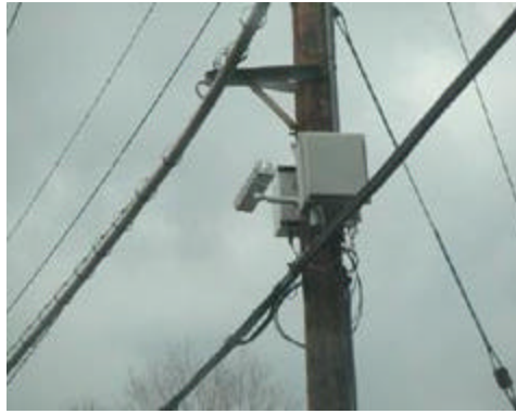
The Briarcliff Manor BPL field trial system incorporates this pole-mounted camera for local authorities to monitor traffic at an intersection near Route 9A. [Alan Crosswell, N2YGK, Photo]
