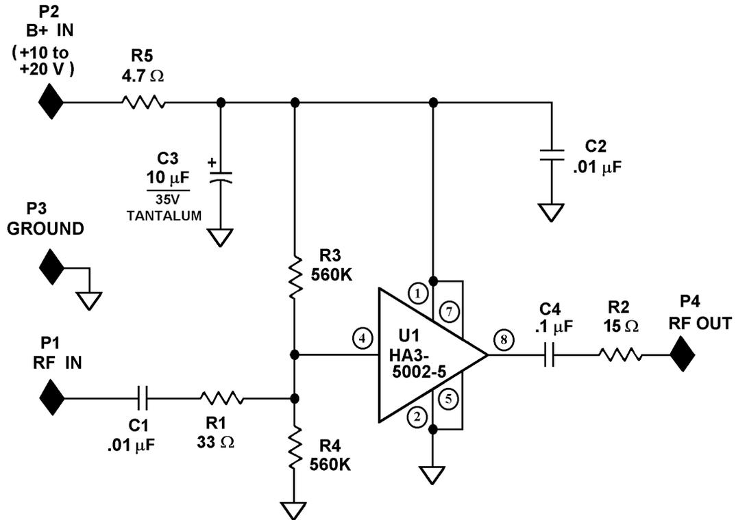
*Figure 3 (above): BUF-F Amplifier Schematic (two per Switch / Amp. Box)*
