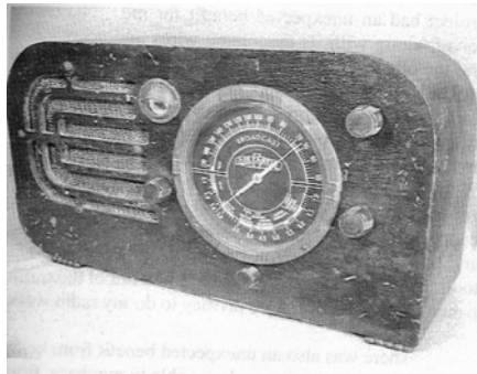
The Air Castle radio. Note the "tuning eye" tube at the upper left of the dial, and the calibrated shortwave scale at the bottom.
