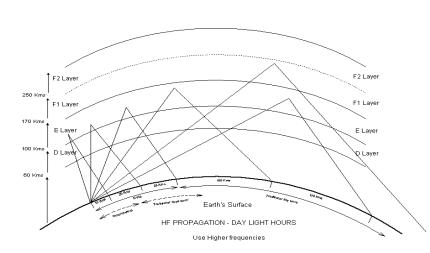
As the signals leave the antennas, they travel up and are refracted off the various ionosphere layers. The lower the signal's incident angle and the higher the layer of refraction, the farther away from the transmitter the signal returns to earth.
