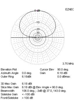
antenna is about 6 db. This over perfect ground. It will be less over actual ground, but ant any rate, the antenna will have a positive gain.
