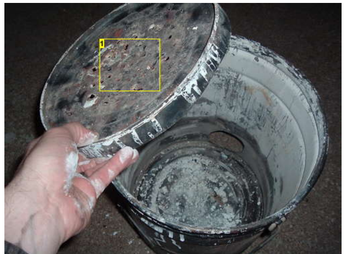
Image Notes 1. punch holes in the center area only to keep the fire focused there.
