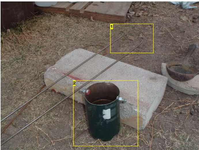
Image Notes 1. hooked tongs for lifting crucible. 2. Crucible made from a camping size propane bottle.
