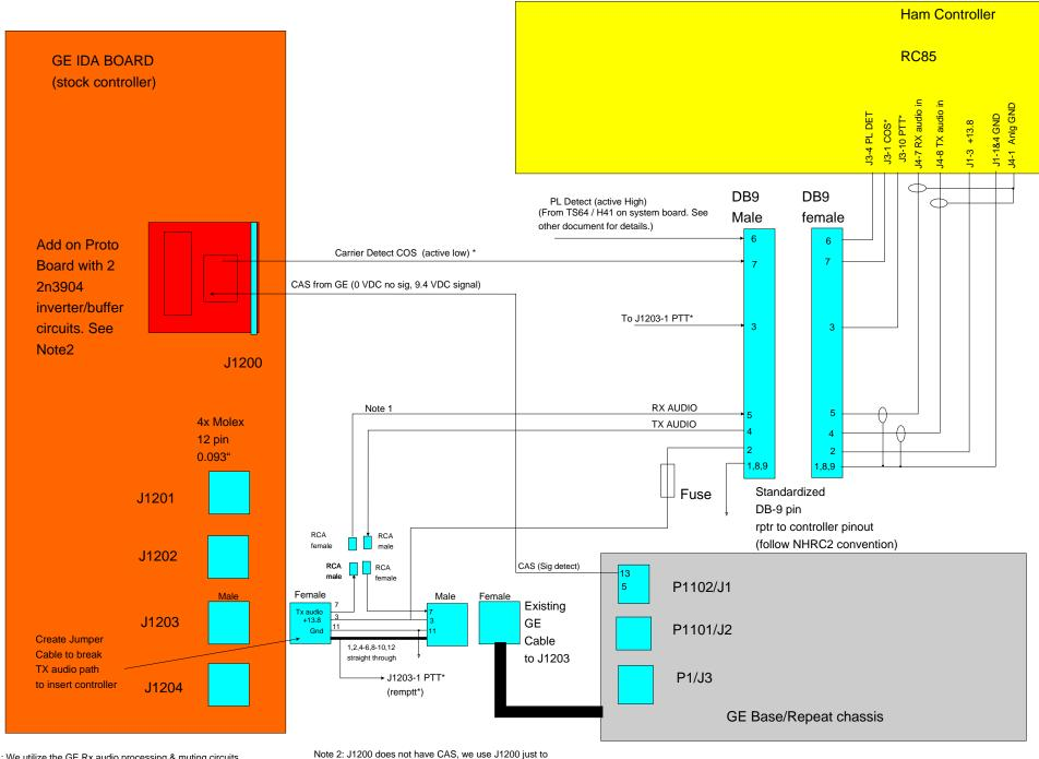
Note 1: We utilize the GE Rx audio processing & muting circuits. We break the regular output toward the tx audio input and feed this into the ham controller as the 'receiver audio'. The ham controllers output is then fed back to the exciter. The break can be re-enabled (by removing jumper cable) to allow the existing controller to act as a backup if the main controller must be serviced.
