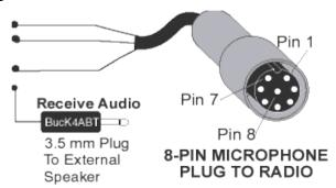
The four (4) signal and control lines associated with PacketRadio I/O are:
