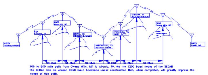
Keyboarding with friends over long distances is easy when using a PacketRadio Network like the South Eastern Digital Association Networks (SEDAN). Very little power is needed, as the nodes along the network perform as "store and forward" devices for this purpose. The nodes do the "store and forward" function automatically. All the PacketRadio user has to do is establish the connection, the rest is handled by the nodes
