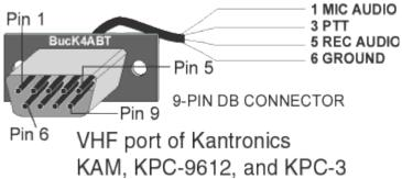
So that we cover other popular radio port interface connector types, the above drawing depicts the VHF radio port of the Kantronics KPC/KAM series. "NOTE that no connections are made to pin 7!"
