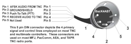
Before we go any further, look at the drawing above; This is one of the most popular TNC (Radio port, Input/Output (I/O)) connectors in use today. This 5 pin DIN connector is almost a "standard of the industry." Knowing the names of the signal and control wires for your TNC will save you a lot of time and grief when making your radio to TNC interface.
