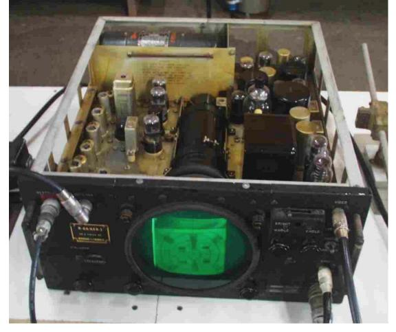
The receiver used to pickup the television signal transmitted by the bomb. A television operator in the controlling plane would tune the signal to give the bombardier a clear picture on his repeat monitor.
