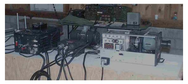
The transmitting equipment that was used during WWII to guide a bomb by television to the target. This equipment was considered to be expendable. On display is the TV camera, junction box, dynamotor, transmitter and antenna.
