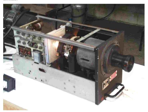
This is the iconoscope television camera, known as a conversion unit. This camera uses the first design of a pickup tube that RCA developed. Normally the lens in the front is more recessed with lock down wing nuts. The lens had to be extended to get a proper focus on an image so close. The camera was designed to have focus at an object at great distance
