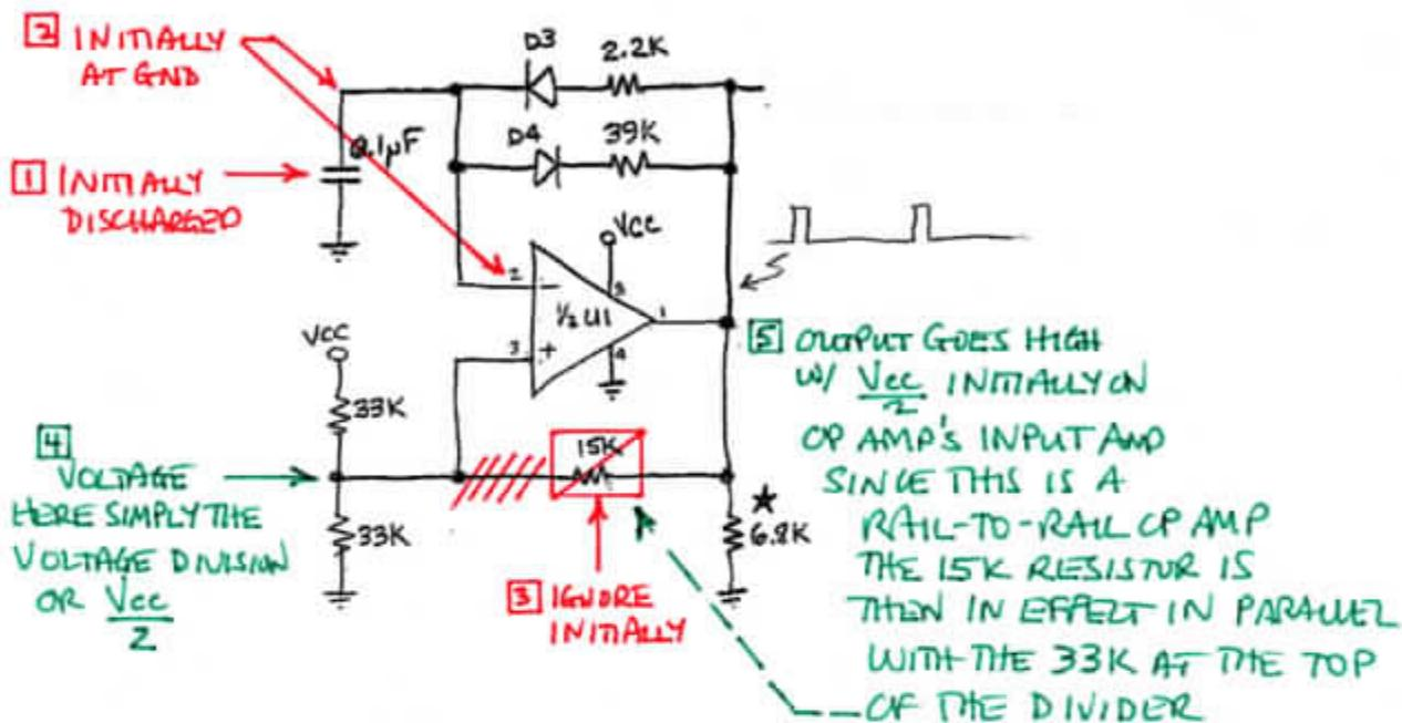
\* NOTE: THIS 6.8K RESISTOR IS NOT NEEDED IF THE OP AMP USED IS A GOOD RAIL-TO-RAIL DEVICE. SOME OP AMPS MAY NEED A PULL-DOWN RESISTOR AT THE OUTPUT TO FUNCTION CORRECTLY.
