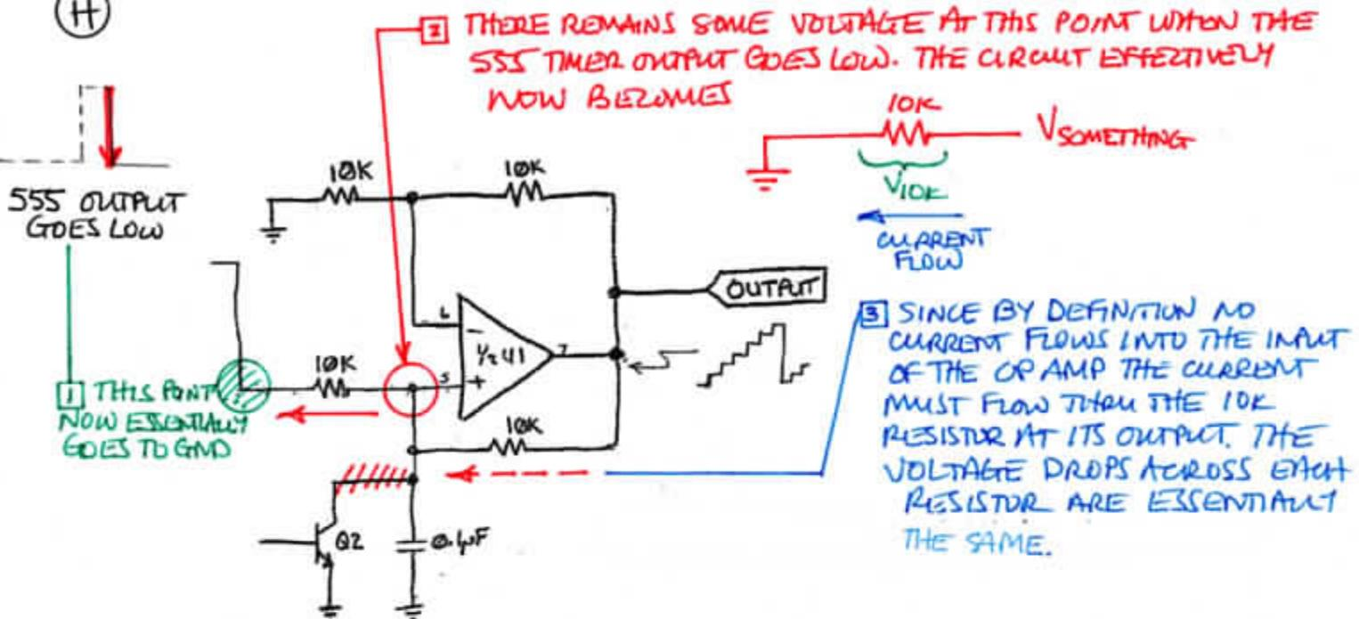
1 WITH THE VOLTAGE AT THE NON-INVERTING INPUT OF THE OP AMP CONSIDERED "X" THEN THE VOLTAGE AT THE OP AMP OUTPUT MUST BE  $\sim 2X$ .
