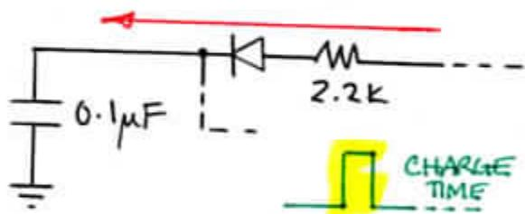
HERE THE CAPACITOR CHARGES MORE QUICKLY SINCE WE'RE GOING THRU A RELATIVELY SMALL 2.2K RESISTOR
