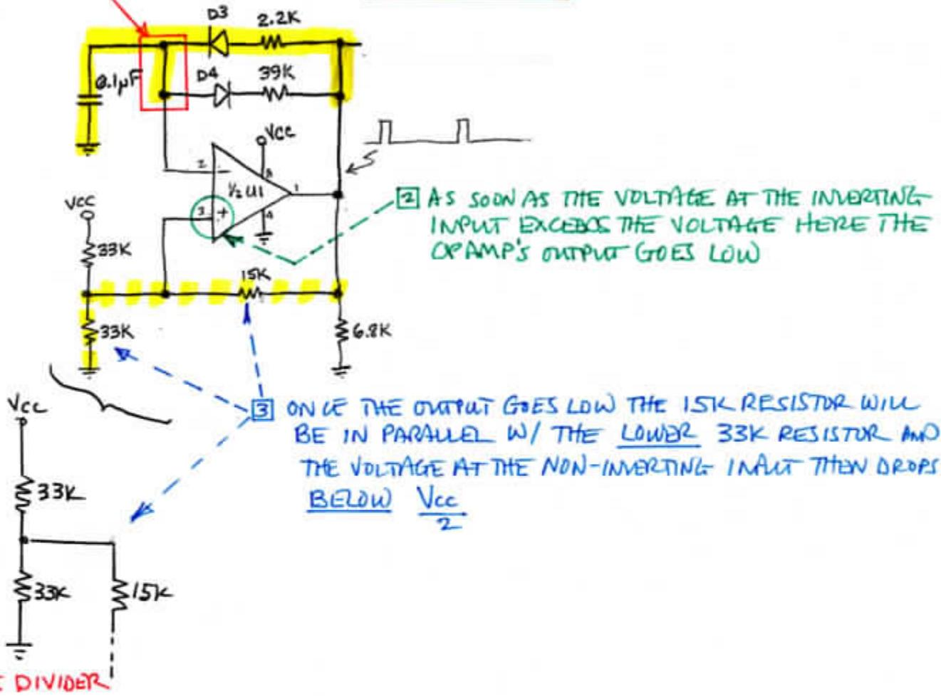
ONCE THE VOLTAGE AT THE INVERTING INPUT (-) BECOMES MUCH HIGHER THAN THAT AT THE NON-INVERTING INPUT (+) [SINCE 15K IS IN EFFECT || TO THE LOWER 33K RESISTOR]
