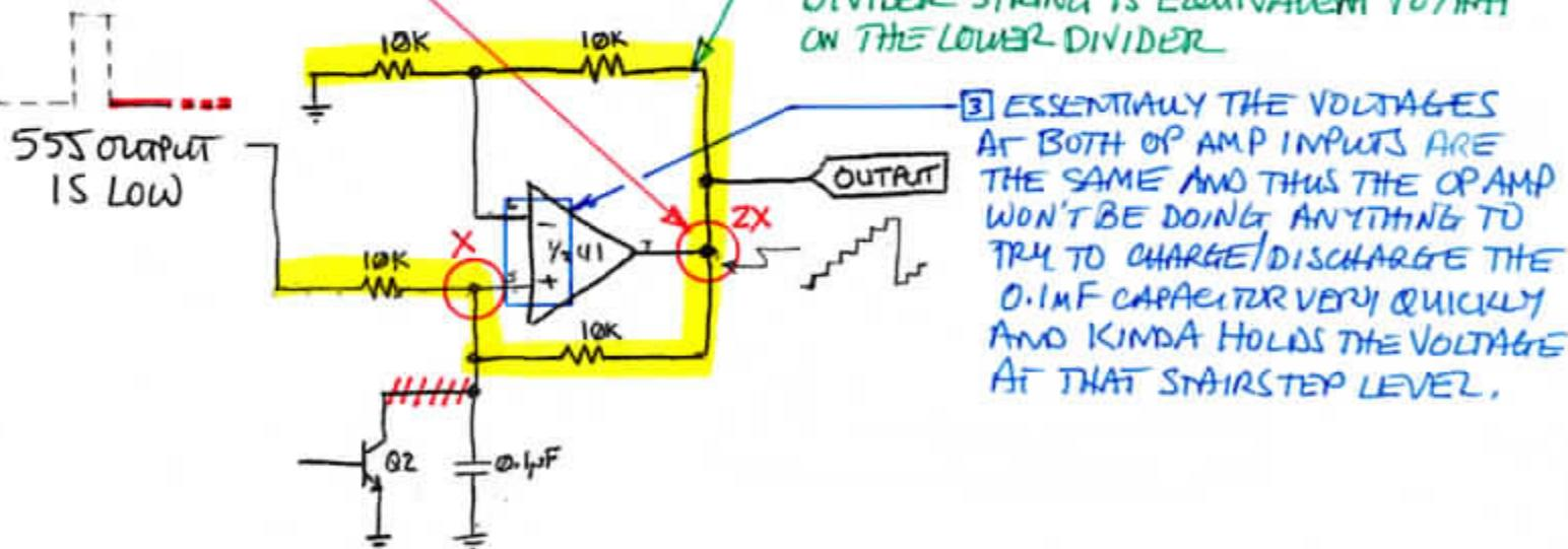
2 SO WHEN THE 555 TIMER OUTPUT IS LOW THE OP-AMP OUTPUT REMAINS STATIC. THERE WILL BE SOME MINOR DROP OFF DUE TO LEAKAGE BUT NOT A SIGNIFICANT AMOUNT.
