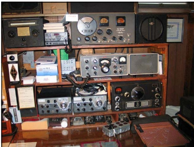
The top radio is a Hallicrafters model SX-25, ca. 1942. In the lower right is a National NC HRO 5TA1 with 13 plug-in coils, ca. 1938.
