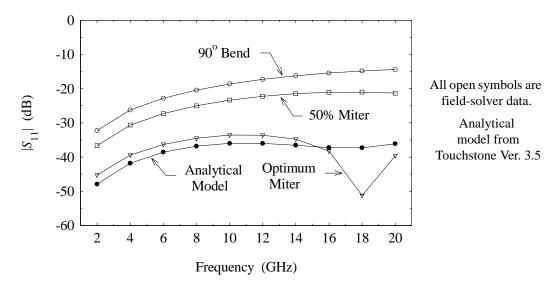
This analytical model seems to work quite well for these substrate parameters and line width. To do a more careful validation, we should also look at the phase responses. Some recent experimental data on the microstrip bend can be found in [26].
