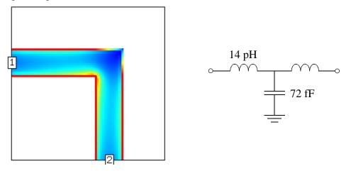
Below the bend has been mitered by 50%. The equivalent capacitance has decreased almost 50% and the series inductance has increased slightly.
