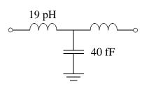
Finally, the "optimum" miter has been computed using a well known formula [25]. The capacitance has been cut in half again and the inductance is two times larger than the full right angle bend case. The current scale is 5-55 amps/meter in all three color plots.
