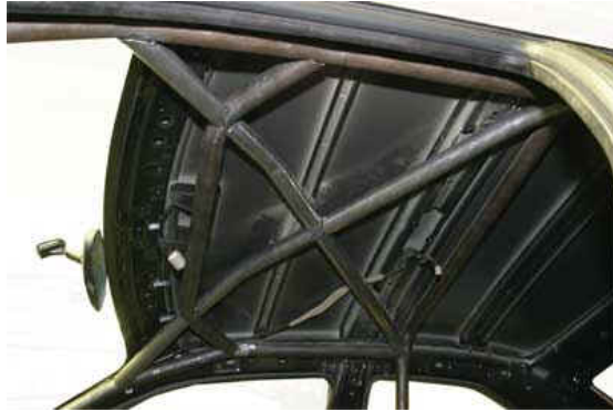
In this photo (Above), the top hoop has been braced (triangulated) and the corner (front of top hoop) has been gusseted with tubes. Notice how the gusset to the A-pillar bar and the top hoop, and the bracing (triangulation) in the top hoop line up. This makes it very strong and also supports the bend.
