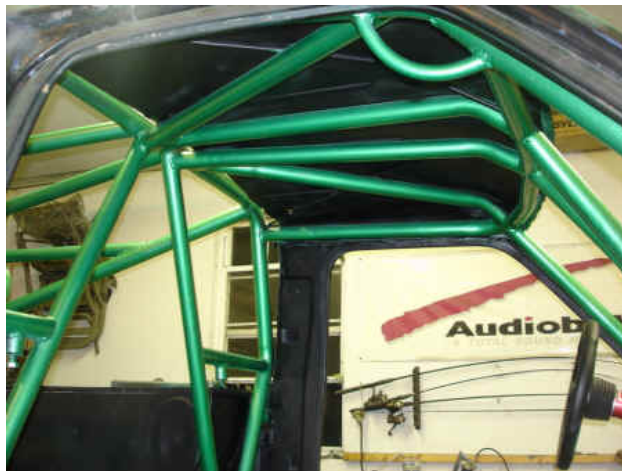
This Bronco II uses a horizontal bar at the bend in the rear B-hoop but cuts it off with a 'A' in the middle. This still provides strength and a point to
