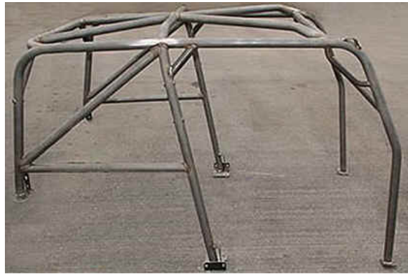
The cage above is from Gen-Right for a Jeep. They've done a nice job triangulating the cage.
