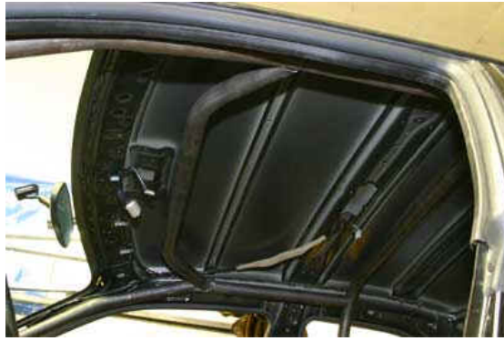
In the photo above is a rear B-hoop, top hoop and A-pillars.
