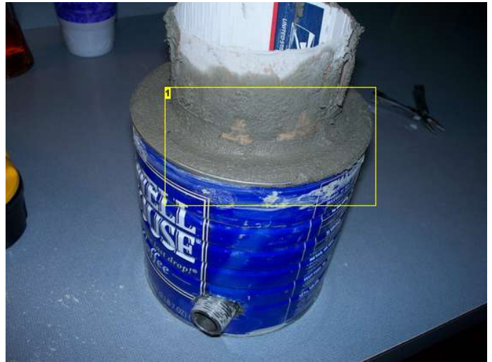
Image Notes 1. put the pipe and cardboard covered can in the can and fill the sides with quickrete. make sure to pack well
