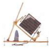
Portable Sun Tracking Solar Panel With A Windup Clock Drive by shastalore
