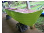
Sailing Canoe Chapter 7: Sew a Skin over the Hull Skeleton and Seal it. by TimAnderson
