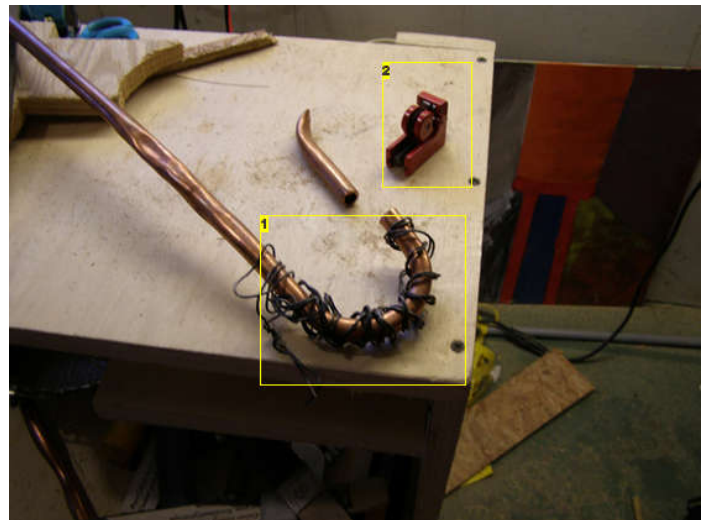
Image Notes 1. Finished bend and extra material 2. pipe cutter
