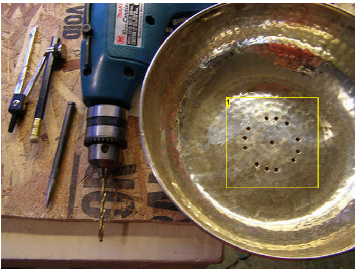
Image Notes 1. Holes drilled for drain
