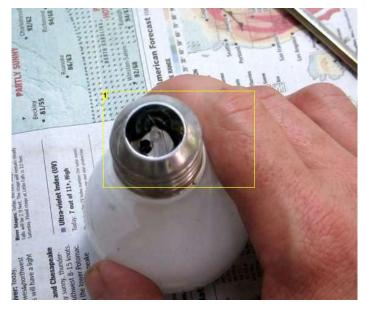
Image Notes 1. Some of the purple glass insulator has been removed. Take the rest out with the screwdriver.
