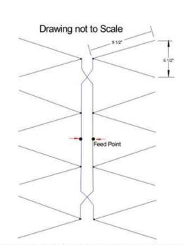
Most any metal will work for the elements. Try to use something near 1/8" diameter and make sure they are free of all coatings and oxidation where they connect to the phase line.
