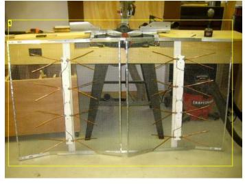
Image Notes 1. Two antennas bolted together with angle iron at the top and bottom to produce and array. This is now a DB8 antenna. One section would be a DB4
