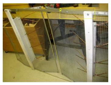
Image Notes 1. Two bolts to connect the angle iron (aluminum) to the antenna. One uses the screw already on the spline the other along the inside of the rail.
