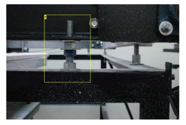
1. The fine adjustment for leveling the machine frame to the movable table.
