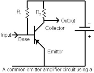
PNP transistor with a single power supply
