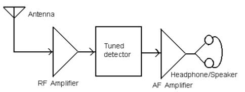
Block diagram of a simple Tuned Radio Frequency (TRF) Receiver
