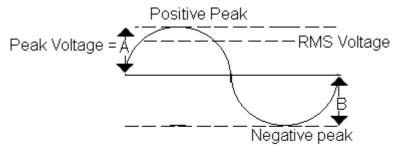
A Sine wave cycle. The upper half denotes the positive cycle and the lower half denotes the negative cycle
