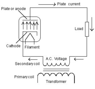
A diode valve as a rectifier
