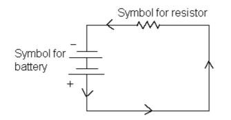
A simple circuit with one resistor and a battery
