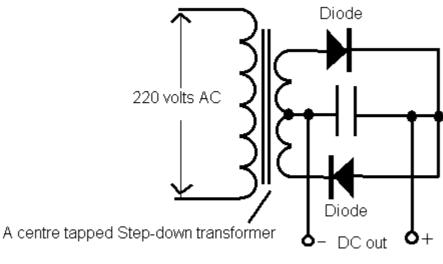
A basic full-wave rectifier circuit
