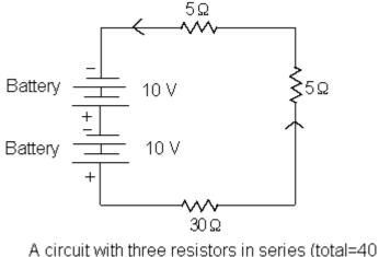
A circuit with three resistors in series (total=40 Ohms) and two batteries in series (total=20 V).
