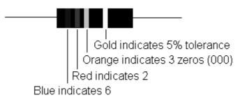
The value of this resistor is 62000  $\,\Omega\,$  or 62 k $\Omega\,$
