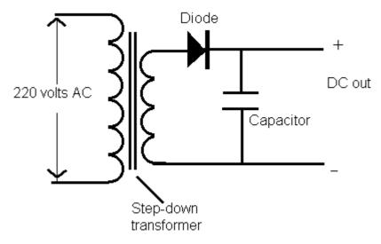
A basic half-wave rectifier circuit
