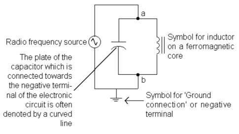
A parallel resonant tank circuit
