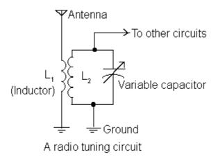
In the tuning circuit shown above, all the frequencies captured by the antenna are passed to ground through the primary coil  $L_1$ . They will try to cause current flow in the tank circuit, but only the resonant frequency will be successful in creating a current flow. The information it carries will be sent to the other radio circuits while the non-resonant frequencies are practically ignored.
