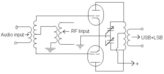
A balanced modulator circuit using valve
