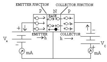
Basic connection of P-N-P Junction transistor
