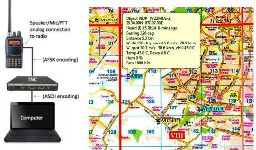
Figure 1: Packet radio stations when use APRS technology, the radio originated information are displayed graphically. In the above figure four radio stations are plotted on a map as per the position information transmitted by these stations. Distance, bearing, time of reporting on map are all automatically archived and available to the radio user.
