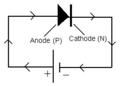
DC Voltage source A forward biased semiconductor diode
