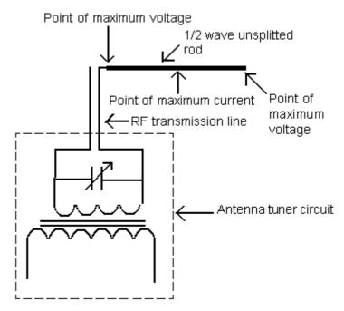
Voltage fed dipole antenna
