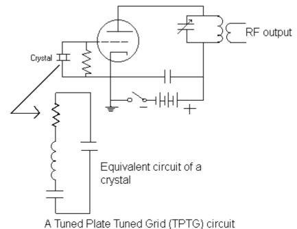
With both crystal and LC circuit oscillating and feeding each other in proper phase, the whole circuit oscillates as a very stable ac source. The plate LC circuit must be tuned slightly higher in frequency than the crystal to produce the required phase relationship between the two circuits to sustain oscillations.
