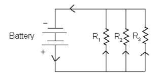
A parallel circuit with three resistors in parallel
