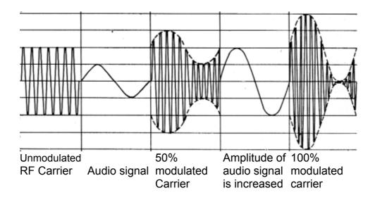
This results in the carrier having two outlines of the audio signal, this is because the variation at instant in the amplitude of the carrier wave is directly proportional to the value of the modulating signal.
