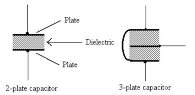
It is seen that a 3-plate capacitor has twice the plate area exposed and thus twice the capacitance.
