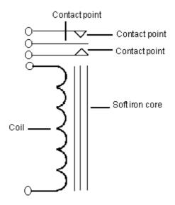
Symbol of an electromagnetic relay
