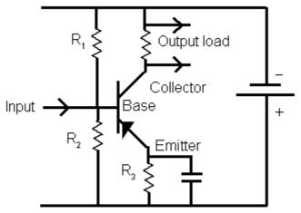
Voltage bias transistor amplifier circuit
