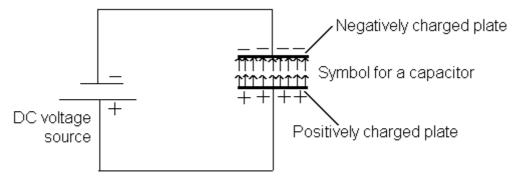
Capacitor in a DC circuit
