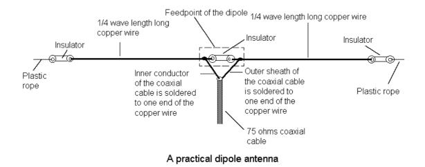
It consists of two straight wire or rod sections, each 1/4 wave long and positioned in one line (collinear). The antenna is fed in the centre by a coaxial cable having a characteristics impedance of 50 Ohms or 75 Ohms.
