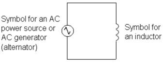
An inductor in an AC circuit
