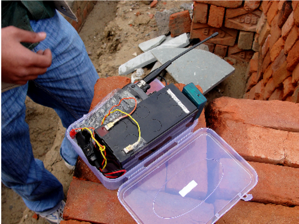
Fox Transmitter with a Pic microcontroller making ready to be hidden beneath a pile of bricks
