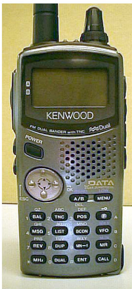
The Kenwood TH-D7 dual-band radio has a built-in TNC and APRS firmware.
