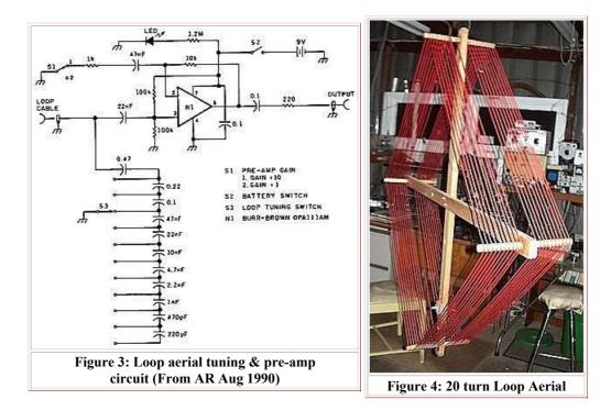
I found that, provided the loop aerial was directed towards the source of signal, the signal received was stronger and less noisy using this loop than using my long wire aerial.
