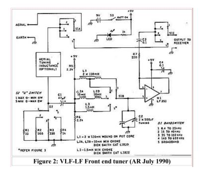
With the RF front end in circuit, minimum discernible signal level is around 3 to 5 microvolta for the regeneration set just below the point of oscillation, At the point of oscillation, the figure is less than 1 microvolt.
