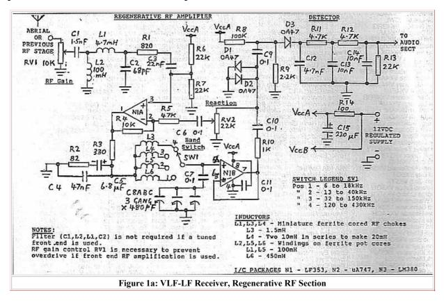
The single tuned circuit is made up of the paralleled sections of 3 gang tuning capacitor C8 and one of the switched inductors L3, L4, L5, or L6. The tuned circuit is connected within the closed loop containing the two amplifiers of an LF353 integrated circuit package. These are JFET amplifiers with a gain-bandwidth product of 4 MHz.
