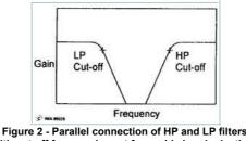
with cut-off frequencies set for a wide band rejection.
