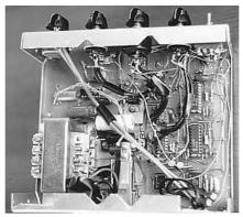
The experimental filter unit with the cover removed.
