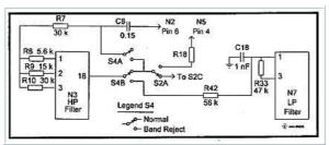
Figure 4 - Changes to the original circuit to include the Band Reject function.
