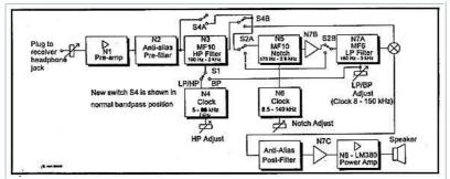
Figure 3 - Block diagram of the Audio Filter Unit with the addition of switch S4.
