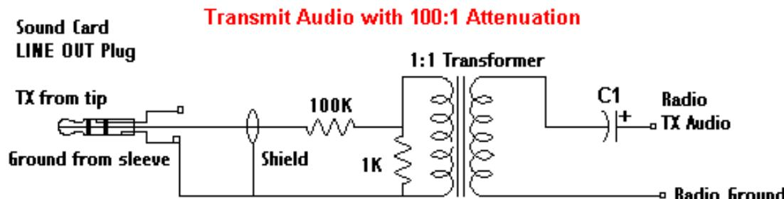
C1 = optional capacitor blocks DC voltage; may be required for radios sharing TX and PTT lines, e.g. hand held radios
