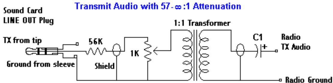
C1 = optional capacitor blocks DC voltage; may be required for radios sharing TX and PTT lines, e.g. hand held radios
