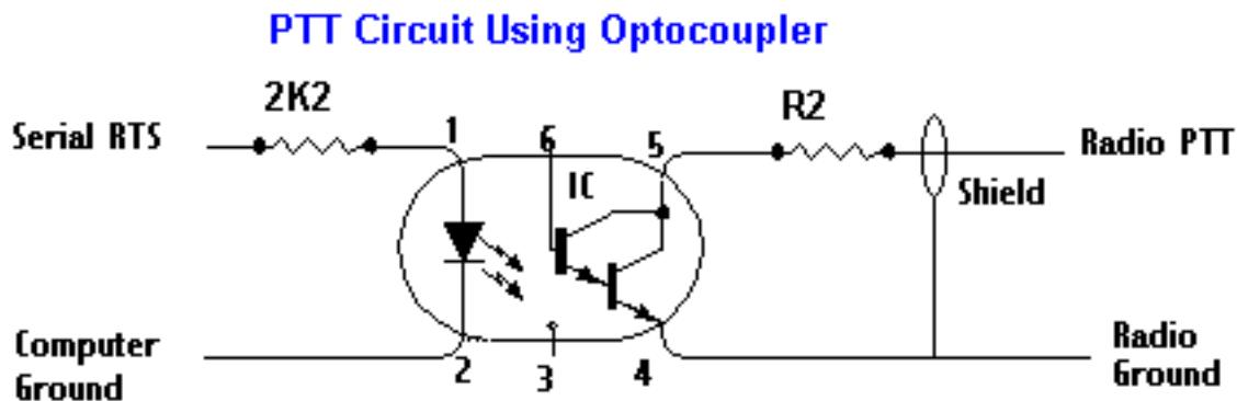
**IC = optocoupler/phototransistor**
