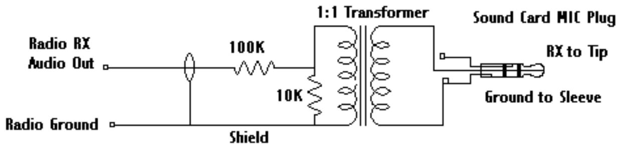
When you're done, tape a "Microphone" label on the sound card end of this RX audio cable so you don't confuse it with the "Line in" or "Line out" cables.
