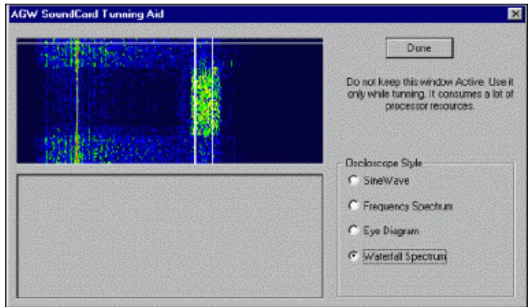
The sound volume (colors) in the **Waterfall Spectrum** can be adjusted by the TX audio volume. But it's better to use the **SineWave** style to see the volume of the incoming signals. The wave heights should only be 1/4 to 1/3 the screen. If necessary, adjust the **Line In** slider in the [Recording window of the Volume Control program](#).
