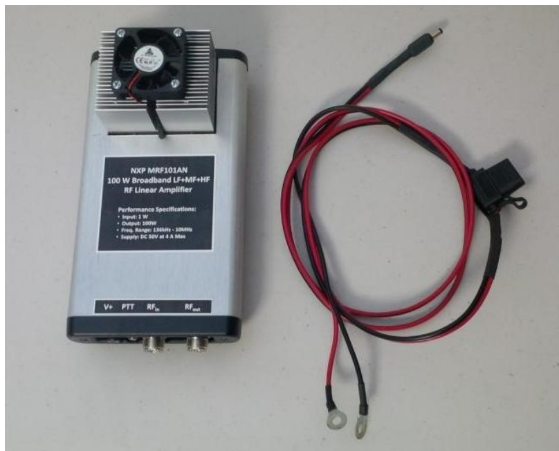
Figure 13: Completed amplifier with fused DC power cable.
