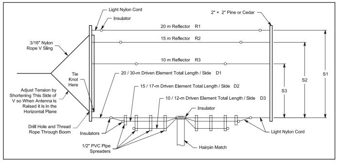
Fig 1—Dimensions for VE7CA's 2-element triband Yagi.
