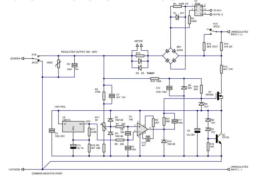
Fig. 11 - Fully-floating 350-400V screen regulator, generating its own +30V rail for the op-amp and voltage reference.
