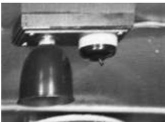
The armless ceiling lamp shown above and right was used in numerous wireless and line communication vehicles and trailers. It had similarities to and might be a modified version of Lamps Operator No. 3
