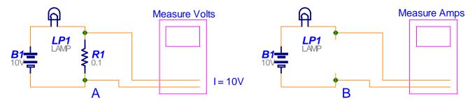
**Experiment:** Using a circuit similar to B above, determine the size of the sense resistor in the multimeter for both the <300mA and <10A settings. You may use a second voltmeter.
