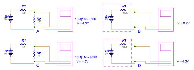
**Experiment**: Use a circuit similar to example D above to measure the input impedance of the multimeter. Adjust R1 until the measured voltage is half of the supply voltage. If the voltage drop is the same then they have to have the same impedance (i.e. the meter input impedance is the same as R1).
