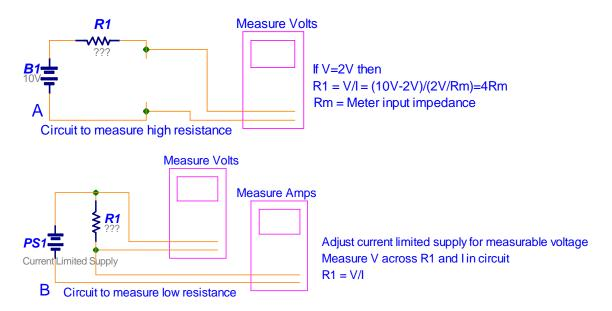
**Experiment:** Measure the resistance of the two items given to you (one is  $\ll 1\Omega$  the other is  $\gg 1M\Omega$ ).
