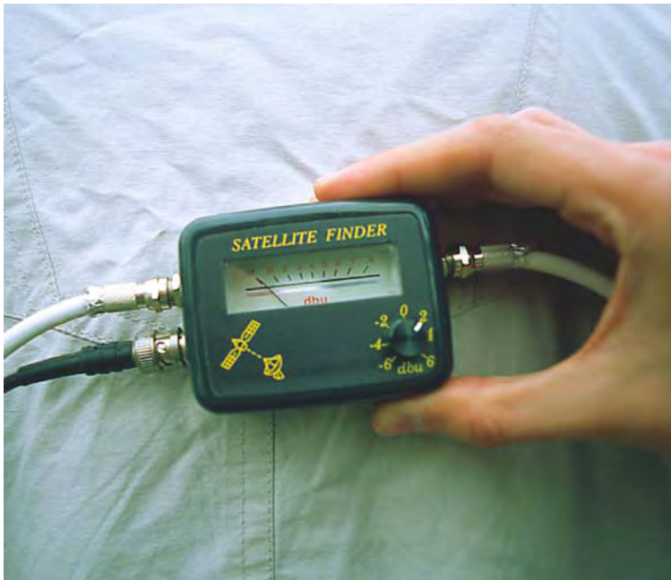
Fig. 5. A satellite finder, such as the Model 3735 from Conrad Electronic shown here, can be easily modified to receive radio-frequency radiation from space. Image courtesy of Peter Wright
