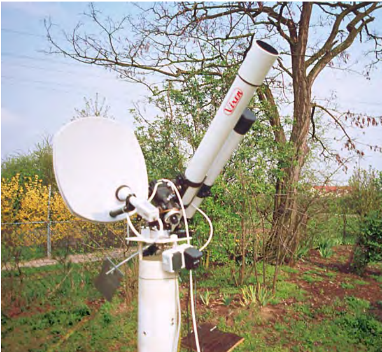
Fig. 7. A satellite antenna mounted in parallel with a telescope enables you to easily track the rotation of the sky. This arrangement also allows for simultaneous observation of an object in the optical and the radio region. Image courtesy of Peter Wright
