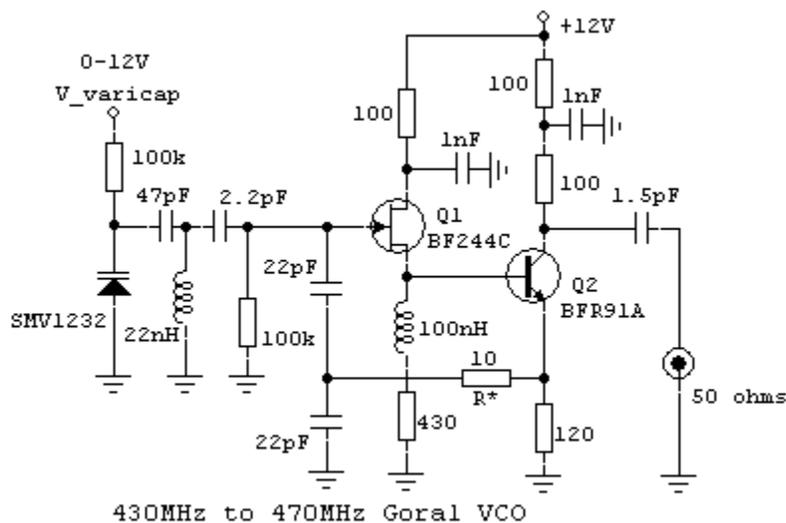
The Goral VCO has an emitter-follower stage inserted in the feedback path of an otherwise conventional Colpitts oscillator circuit.
