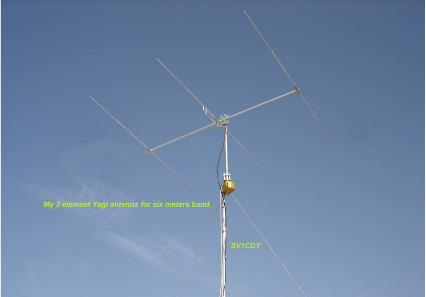
This is another on tree elements Yagi-Uda antenna, based at same computing formula but this time for six meters band.
