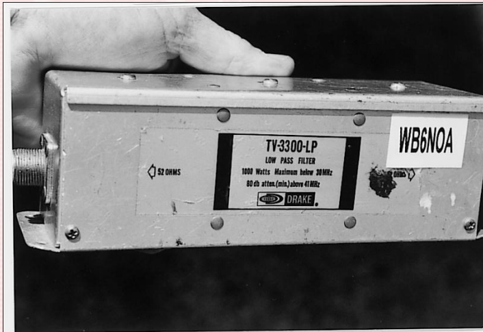
Drake TV-3300-LP Low Pass Filter. 80 db attenuation above 41 MHz. 1000 Watts below 30 MHz.
