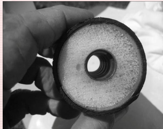
Large coax, with hollow center conductor, low loss
