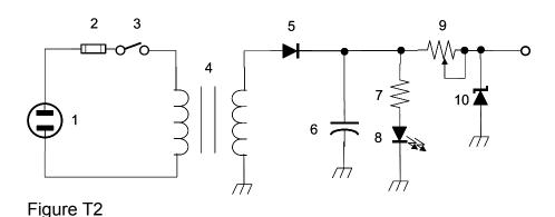
The circuit shown in Figure T2 is a simple power supply. Component 2 is a fuse. Item 3 in figure T2 is a **single-pole single-throw** switch. (T6D03) It turns the power supply on and off.
