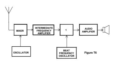
The type of receiver shown in Figure T6 is a **single-conversion superheterodyne receiver**. (T7A02) The function of a mixer in a superheterodyne receiver is to **shift the incoming signal to an intermediate frequency**. (T7A03) The function of a product detector (block #1 in Figure T6) is to **detect CW and SSB signals**. (T7A01)
