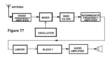
The block diagram for an FM receiver is somewhat different than the block diagram for a superheterodyne receiver. If block 1 in Figure T7 is a frequency discriminator, the circuit pictured is **an FM receiver**. (T7A04) A **discriminator** is the circuit that demodulates FM signals. (T7A11)
