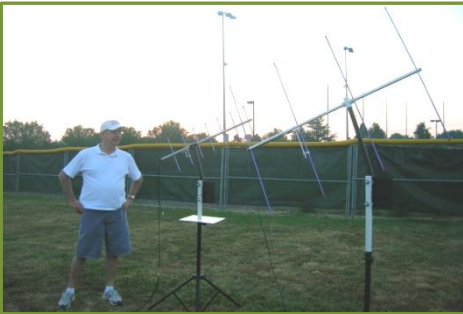
Satellite communications antennas.
