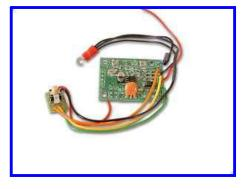
The BHI NEDSP1061-KBD module (originally built for the YAESU FT-817 and the KENWOOD TS-50) can be used with the same great results on a YAESU FT-897D.
