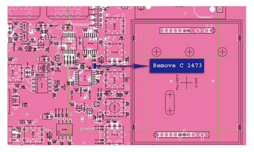
2. Add a capacitor at the output of DSP module! (10-100 nF). Why to add a capacitor? To isolate the DC voltage found at the input of the M51132FP IC from almost grounded DSP module output). I used a 10nF capacitor found in my stash.
