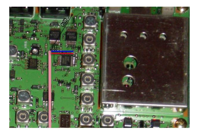
5. Solder the red (power) lead to the drain of Q 1014
