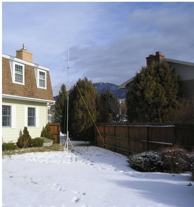
Hustler 4-BTV antenna temporarily installed in side yard. Note location of guy ropes from spider assembly near top of antenna to the ground.
