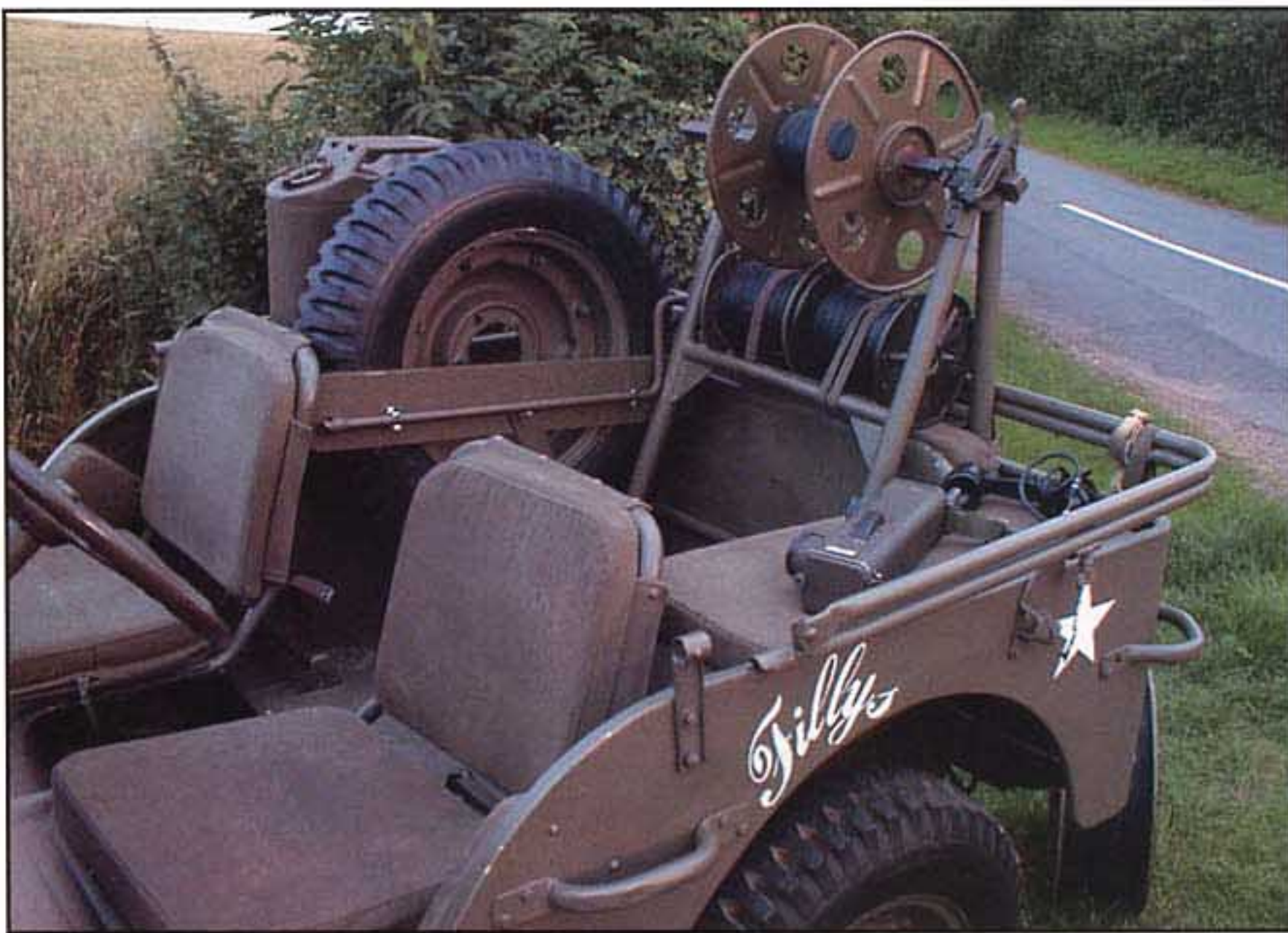
RL-31 unit mounted on the Jeep. The hand clutch/brake mechanism can be clearly seen and is used for slowing the drum when paying out cable. Also shown on the rear seat are the BC-611 Handie Talkie radio and TS-10 sound powered handset which would be used when testing a new cable installation. The web strap holding down the passenger seat can be seen fitted as per the tech manual.
