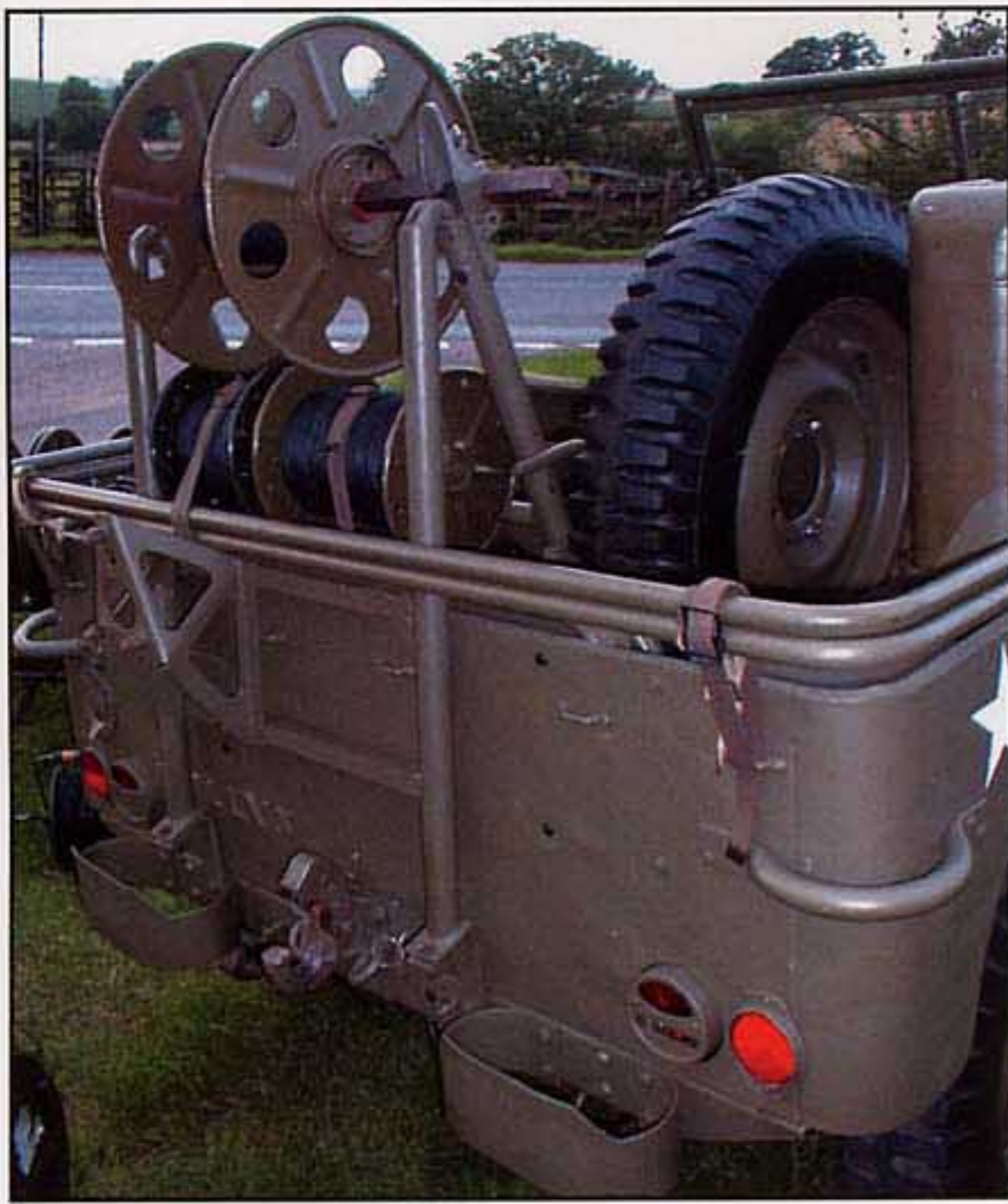
Rear view of the RL-31 unit mounted on the Jeep. The gas can and spare wheel are mounted inside the vehicle so as not to interfere with cable laying. The spare wheel carrier is shown mounted onto the rear of the RL-31. This is a non-regulation field mod – in practise if the carrier remains attached to the spare wheel as described in the TM it interferes with access to the rear tool box.
