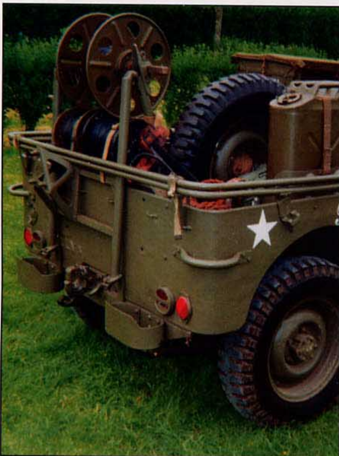
View showing the rear of the Willys MB with the mounting brackets that support the RL-31. These were field manufactured, and are bolted to the rear cross member. The reel is positioned offset from centre allowing for the spare wheel to be located on board as per the regulation.
