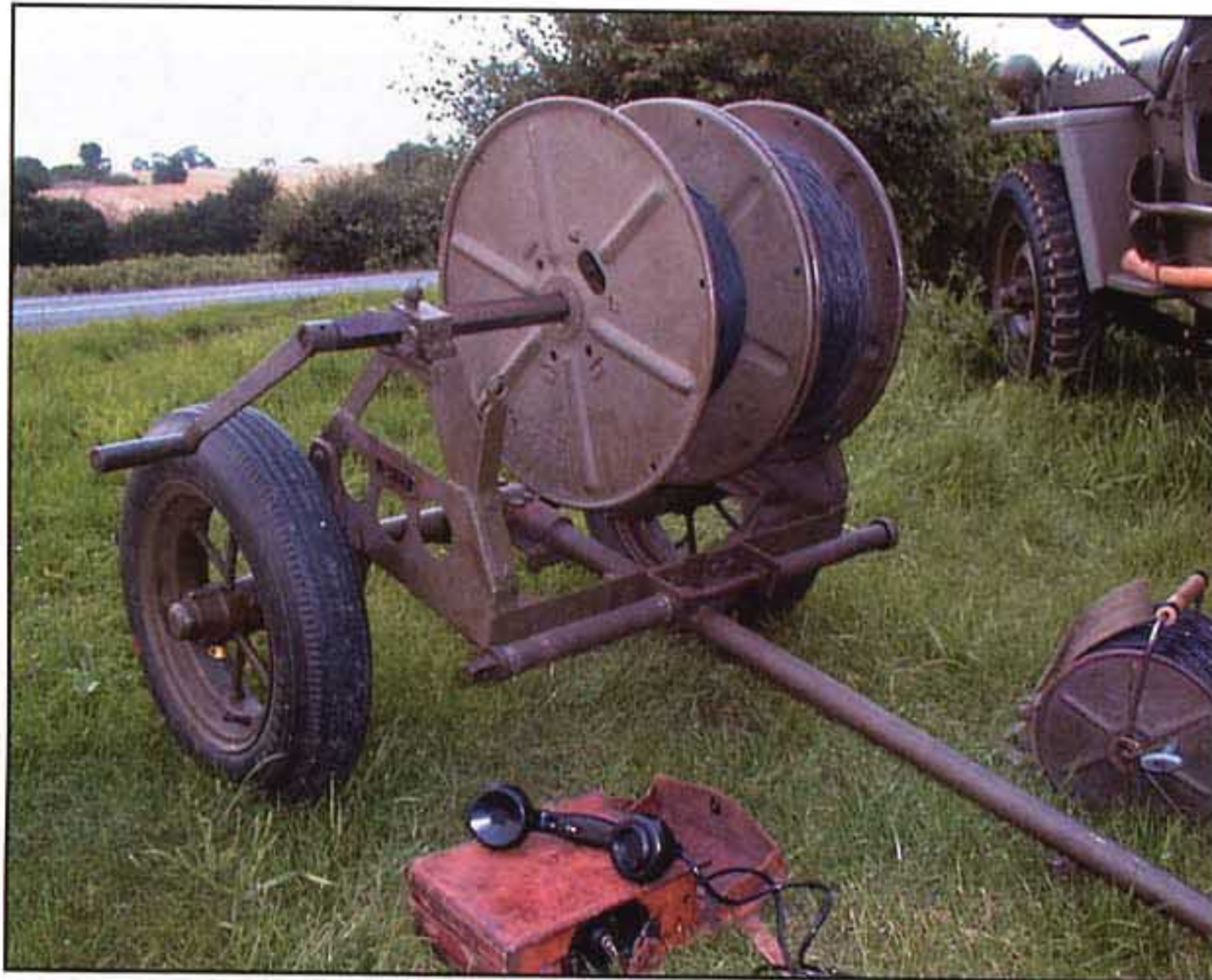
Close up detail of the RL-35 cable cart. The hand reel spindle can be seen fitted to the front of the cart in its stored position. The spare winding handle is located under the reels on the cart. Laying beside the cart are the EE-8A field phone and DR-8 cable drum.
