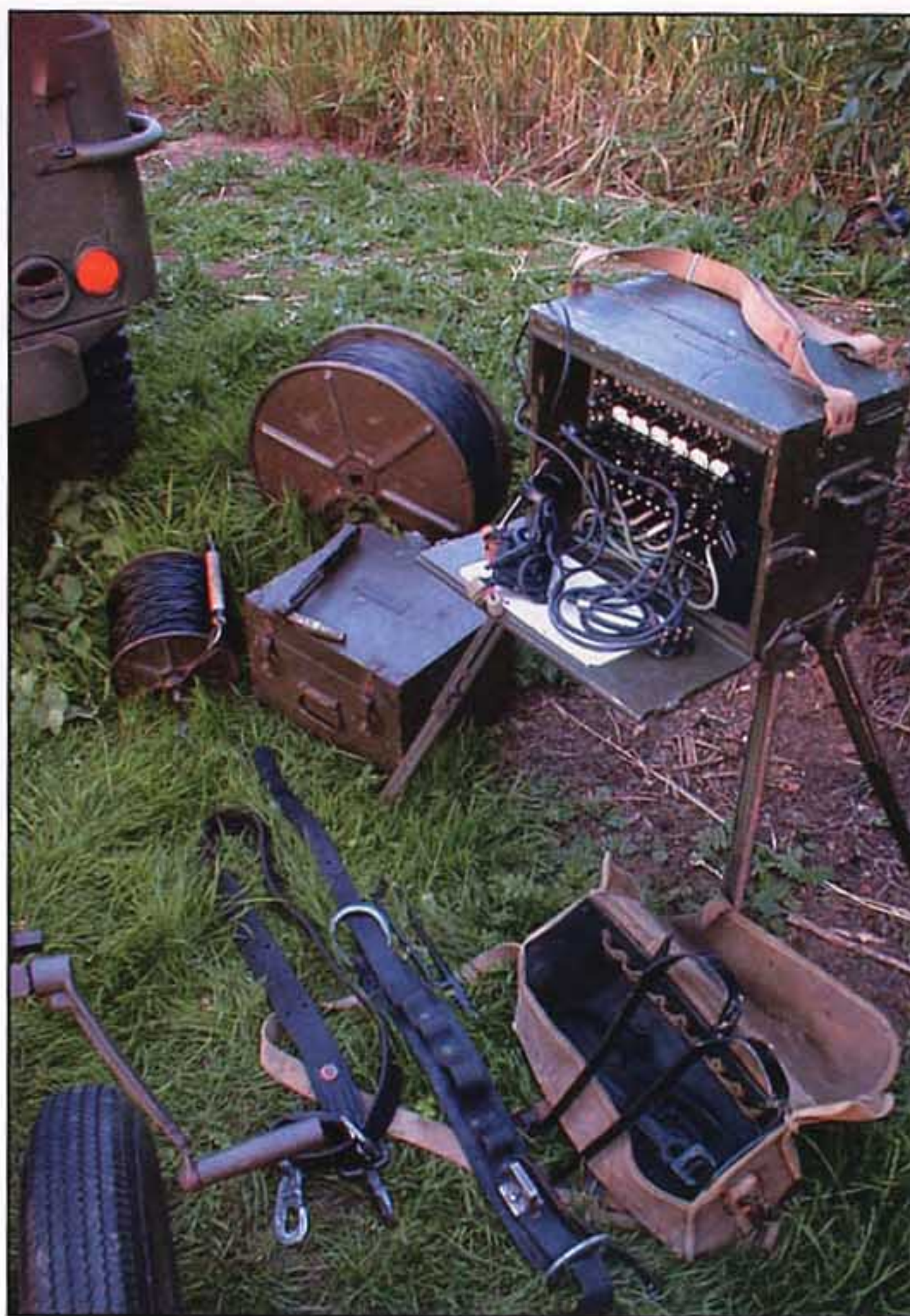
BD-71 six line field exchange (switchboard) pictured with lineman pole climbing belts and spurs (leg irons) The RL-35 cable trailers tire tread pattern detail can be seen here.
