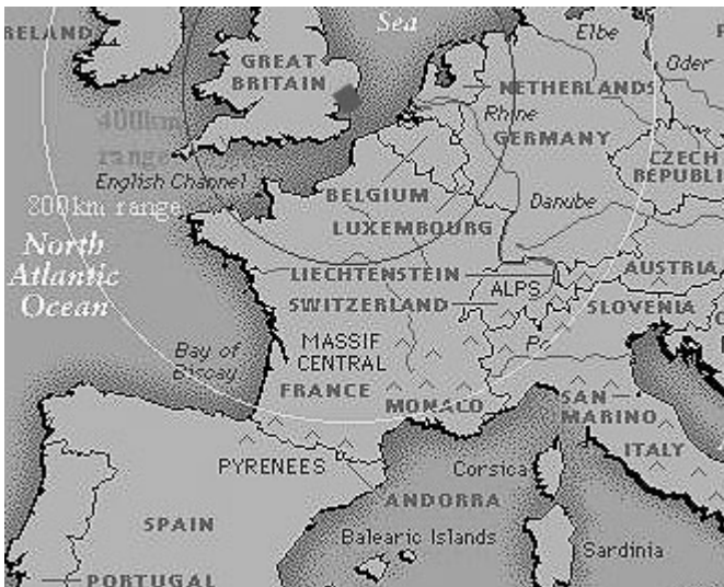
Fig 3. Approximate 400km and 800km range map for rain scatter communications from grid JO02 in the UK.
