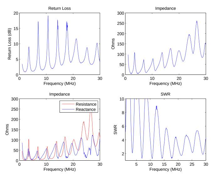
The SWR minimum is very narrow as the half-wave resonances. Between the resonances, the SWR remains above 6:1-8:1 (400  $\Omega$  to 600  $\Omega$  antenna impedance). At the higher bands, the impedance of the wire increases even in between the resonances, resulting in better matching at the half-wave resonances and in between the resonances. However, there still is probably some decrease in the SWR due to loss in the ferrite.
