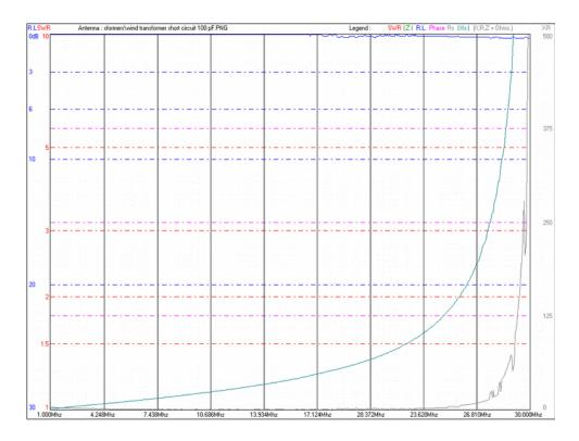
Short circuit reactance of the transformer including a 100 pF capacitor across the primary.
