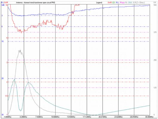
Open circuit reactance of the transformer. With  $L_I = 0.3 \ \mu\text{H}$  leakage inductance, for series resonance to occur at  $f_R = 18$  MHz, the secondary winding capacitance is  $C_s \approx N_p^2 / (8\pi^2 N_s^2 L_I f^2)$  or 2 pF.
