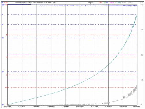
The short circuit test indicates 57  $\Omega$  ohms of impedance at 10.68 MHz which corresponds to 0.85  $\mu$ H leakage inductance.
