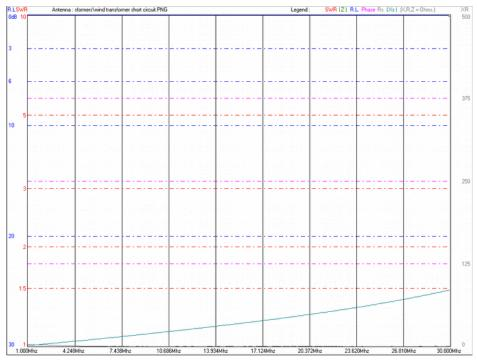
Short circuit reactance of the transformer. To calculate the leakage inductance, at a frequency well below the self-resonance frequency, such f = 10 MHz, observe the reactance, which in this case is approximately  $X = 20 \ \Omega$ . Then the leakage inductance  $L_I = X/(2\pi f)$  or approximately 0.3  $\mu$ H.
