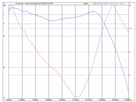
Back-to-back transformer test with 8.0 µH of inductance in series between the two secondaries of the transformers. Resonance occurs at about 22 MHz with about 1 dB loss per transformer.
