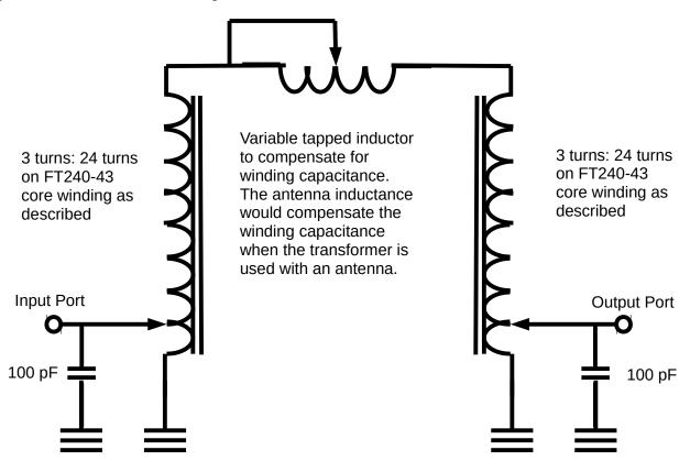
As the inductance between the two transformers is increased, the winding capacitance is resonated at a lower frequency. At the resonant frequency, the winding capacitance is an open circuit and therefore does not degrade the impedance transformation.
