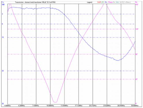
Back-to-back transformer test with 33.3 µH of inductance in series between the two secondaries of the transformers. Resonance occurs at about 10 MHz with about 0.5 dB loss per transformer.
