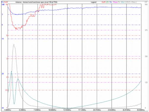
Open circuit reactance of the transformer with  $C_p = 100 \text{ pF}$  across the primary. The new resonant frequency is  $f = \left[8\pi^2 \left(C_s N_s^2/N_p^2 + C_p\right) L_I\right]^{-0.5}$  or 13.6 MHz as predicted.
