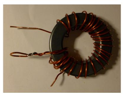
This uses a more conventional winding technique with 3 turns of primary and secondary that are twisted together, and 21 more turns of separated secondary winding.
