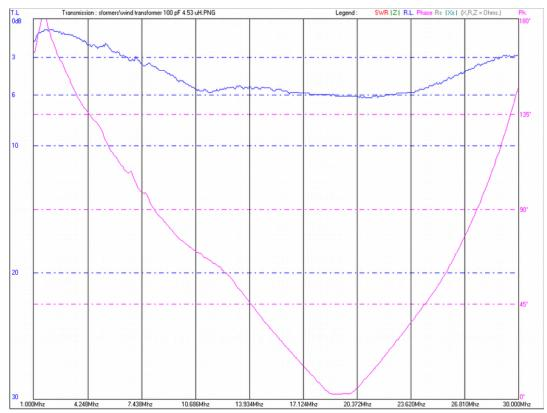
Back-to-back transformer test with 4.5 µH of inductance in series between the two secondaries of the transformers. Resonance occurs at about 30 MHz with about 1.5 dB loss per transformer.
