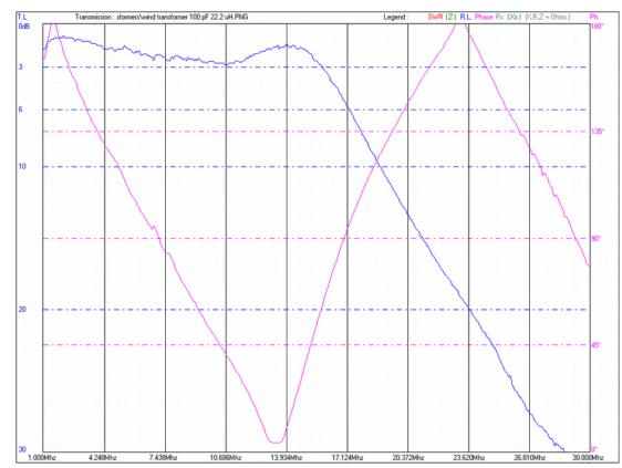
Back-to-back transformer test with 22.2 μH of inductance in series between the two secondaries of the transformers. Resonance occurs at about 14 MHz with about 0.75 dB loss per transformer.
