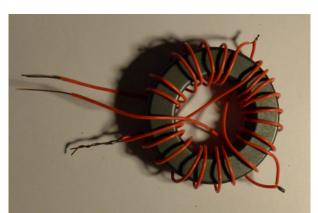
Twist end of fourth wire on the beginning of the first coil, looping over the toroid. Twist the end of the first coil on the beginning of the second coil, looping over the fourth wire. Finally, twist the end of the second coil onto the third coil, looping over the fourth wire again. The four wires together make 24 loops over the core. When you are done, solder the twisted wires together. Keep the wires spaced apart, make sure they do not touch!
