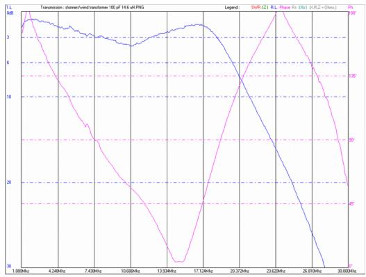
Back-to-back transformer test with 14.6 μH of inductance in series between the two secondaries of the transformers. Resonance occurs at about 16 MHz with about 0.75 dB loss per transformer.
