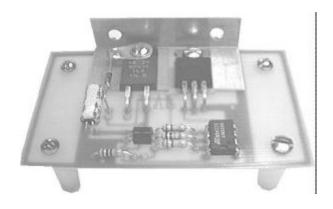
Fully-constructed unit before attachment to a Gunn source. Please note the placement of the 1N914 diode for heat-sensing, and note that the solder-lug is firmly attached to the top-side of the heater resistor. The heater resistor itself is firmly seated on the metal bracket to transfer heat and warm the bracket. The transistor is mounted using an insulated shoulder-washer and an insulating sheet, so that it has no electrical contact with the metal bracket.
