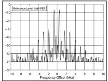
Figure 1—Spectral display of the TS-570S(G) transmitter during two-tone intermodulation distortion (IMD) testing on 6 meters. The worst-case third-order product is approximately 32 dB below PEP output, and the worst-case fifth-order product is approximately 35 dB down. The transceiver was being operated at 100 W output at 50.2 MHz.
