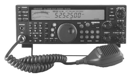
mode band coverage (25 W AM) from 160 through 6 meters and an extended general coverage receive range of 0.5 to 60 MHz. The built-in antenna tuner also works on 6 meters, and comes in very handy for matching a single 6-meter antenna across the relatively wide 4 MHz range between 50 and 54 MHz. The tuner is also effective for employing a number of antennas intended primarily for HF, such as 40 and 80-meter dipoles for example, on 6 as well.
