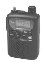
ranging from 5 kHz to 100 kHz—including a 6.25 kHz setting—are independently selectable for each band. An RIT function for use above 835 MHz is also included.
