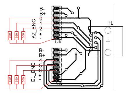
This solution was tested with some bad cables and fixes the problem 99% of the time; this problem was present only one time on the field but represents a good solution if somebody has the same problem. We test also with 1.2K ohms but in the case of Gerard the unstable lectures back, depending how noisy is your antenna place you need to try with values from 470 ohms to 1.5K ohms.
